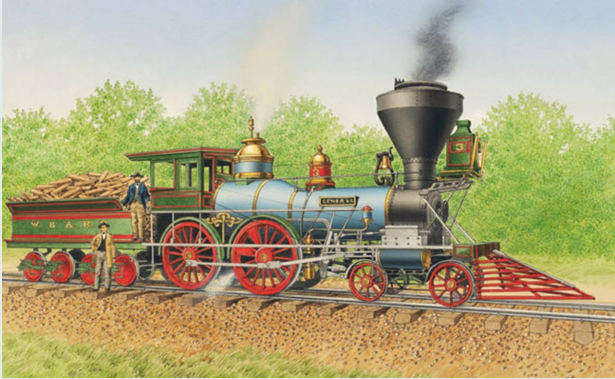
The General , a 4-4-0 "American" type steam locomotive
