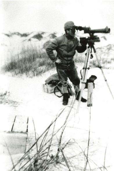
Left, a soldier of the 244th Coast Artillery using an azimuth telescope at Fort Macon in 1942. Below and right, the telescope mounted and ready for use.
